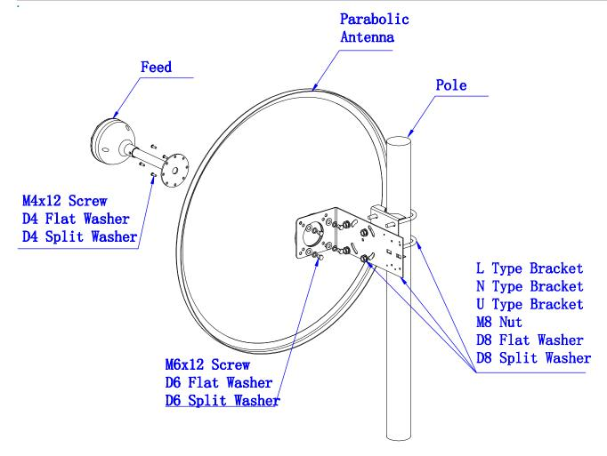
Click the following link (or enter part number in "SEARCH" on website) to obtain additional part information including price, inventory and certifications: 3300-4200 MHz, 2-Foot, 24 dBi, Parabolic Dish Antenna, Vertical/Horizontal Polarized, 2 x N-Type Female Connectors KP-35PD2-N-V2
