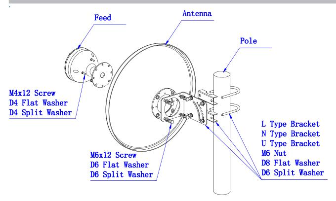
Click the following link (or enter part number in "SEARCH" on website) to obtain additional part information including price, inventory and certifications: 3300-4200 MHz, 1-Foot, 18 dBi, Parabolic Dish Antenna, Vertical/Horizontal Polarized, 2 x N-Type Female Connectors KP-35PD1-N-V2
